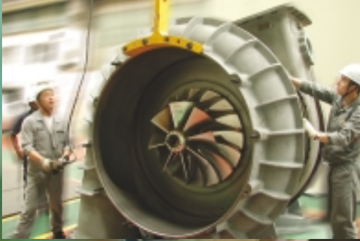
Engine air outlet being fitted
