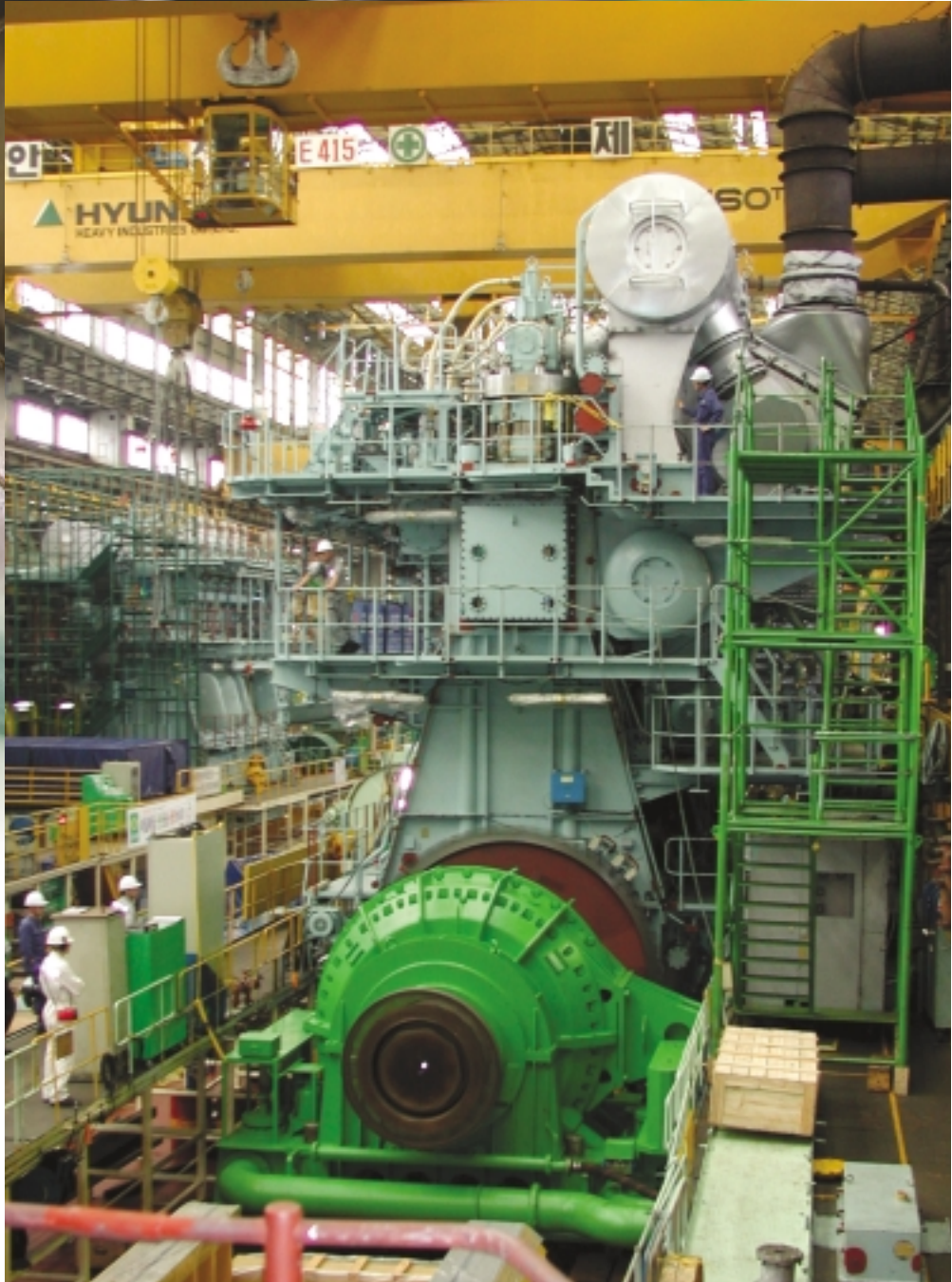
Low speed diesel unit D15 being tested at the Hyundai plant in Ulsan, South Korea
